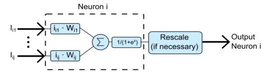
In this case, the proposed network has a structure of nine neurons in the input layer (one per input), three neurons in one hidden layer, and one neuron in the output layer. The output neuron offers as output an estimation of the weight of the studied animal that produces the evaluated pattern. This neural network is depicted in Figure 4.
