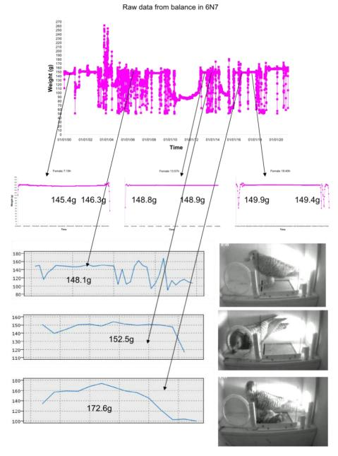
In our results, stable patterns, due to the tare and gain calibration, offer weight estimation with accuracy better than a gram. As can be seen, the system offers an error in the range predicted by the
