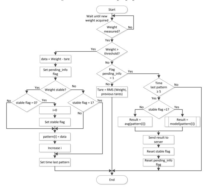
**Figure 1.** Flow chart of the weighing algorithm.
